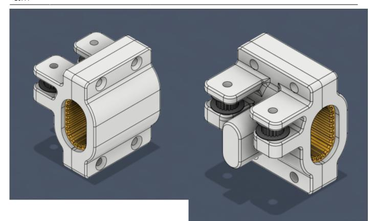
Then created some bearing holders with idler pulley holders and mounts for the cross bar.
