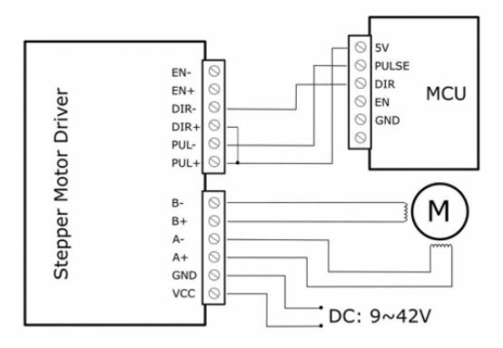
So in keeping with the proposed vendor Microcontroller wiring we then add the enable lines back in and it should look like
