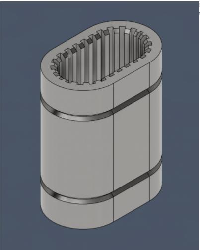
l created some oval shaped linear bearings for starters and testing them on the rails.
