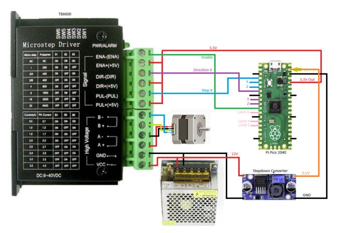
This schematic show the wiring for the X axis, the two Y axis connections for direction and step should be used instead.
