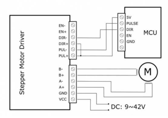
So in keeping with the proposed vendor Microcontroller wiring we then add the enable lines back in and it should look like this.
