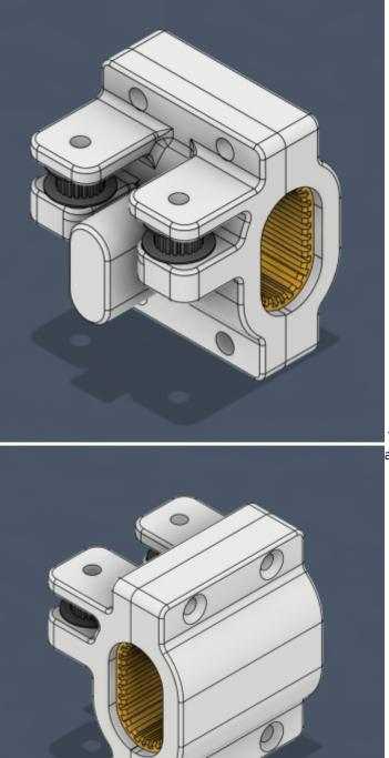
Then created some bearing holders with idler pulley holders and mounts for the cross bar.
