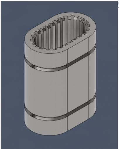
I created some oval shaped linear bearings for starters and testing them on the rails.
