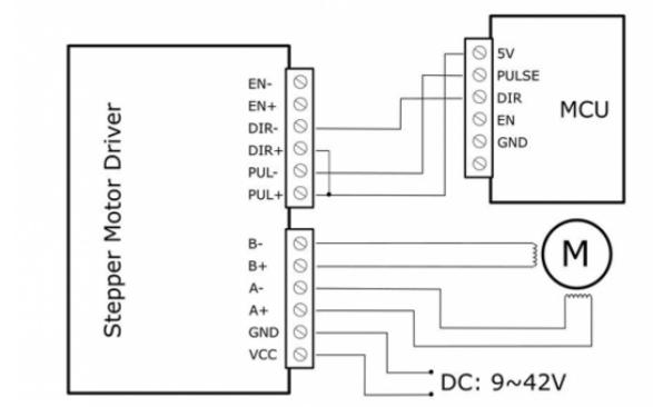
So in keeping with the proposed vendor Microcontroller wiring we then add the enable lines back in and it should look like this.
