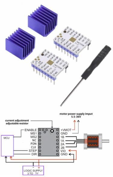
So some further research had some reasonably costed silent steppers and I opted for some TMC2208<sup>14)</sup> drivers from Amazon and tested then out. I got two for around €9.00, and wired up a motor to a pico 2040 and proceeded to do some tests.
