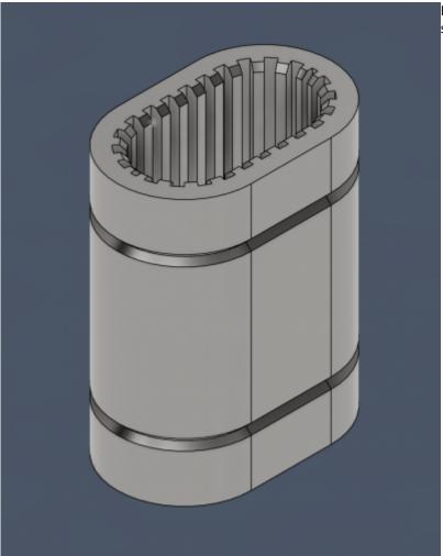
l created some oval shaped linear bearings for starters and testing them on the rails.
