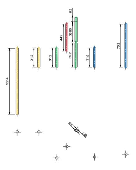
The bearings selected for this project has a 4mm inner diameter, so the shafts to be prepared is 4mm thick and of various lengths as show in the diagram above.
