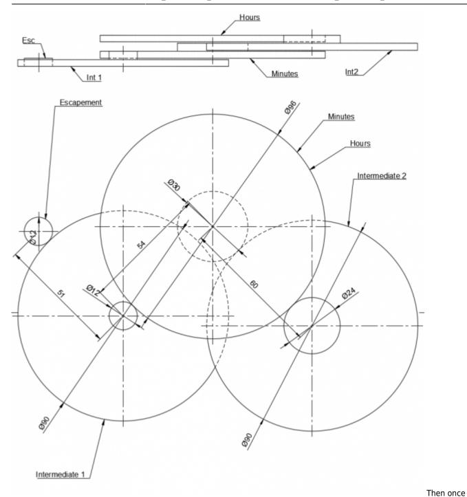
the dimensions were determined I simply rotated the entire geartrain into a zig-zag patters with 45 and 90 degree angles, resulting in this compact layout.
