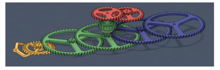
So this is a coloured view of the entire drive train with the yellow parts being responsible for generating the seconds, green then stepping that down to minutes and delivering the output to a shaft driving the minute hand. The red gears than steps everything down further by a combined ratio of 12 and driving the hour hand. Lastly the blue gears stepping down everything by another ratio of 56.25 to provide enough power for 10 days.
