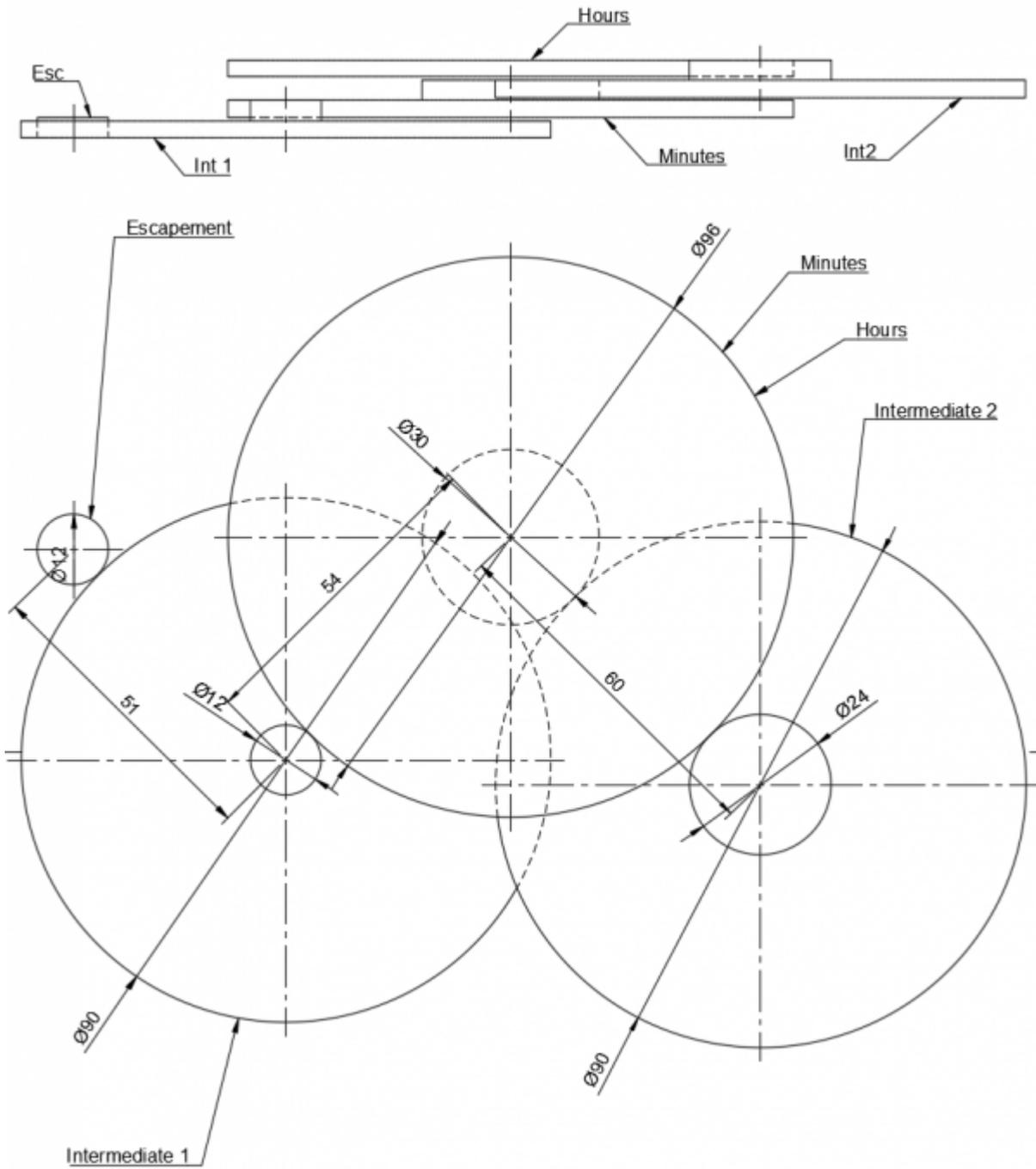
Then once the dimensions were determined I simply rotated the entire geartrain into a zig-zag pattern with 45 and 90 degree angles, resulting in this compact layout.
