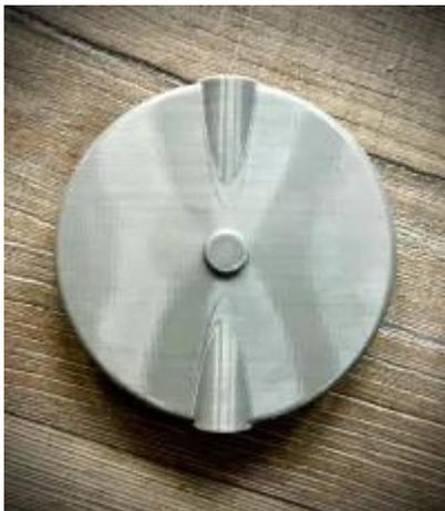
The [pendulum weight design](#) is 100mm in diameter and hollow and filled with sand to create the weight. The design linked here fully filled is about 140g.
