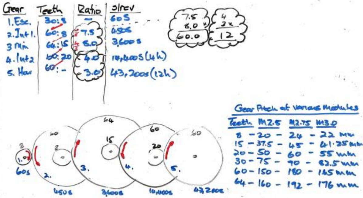
Combining whiteboard designs and sketching using fusion I managed to figure out a layout and some ratios that can work.
