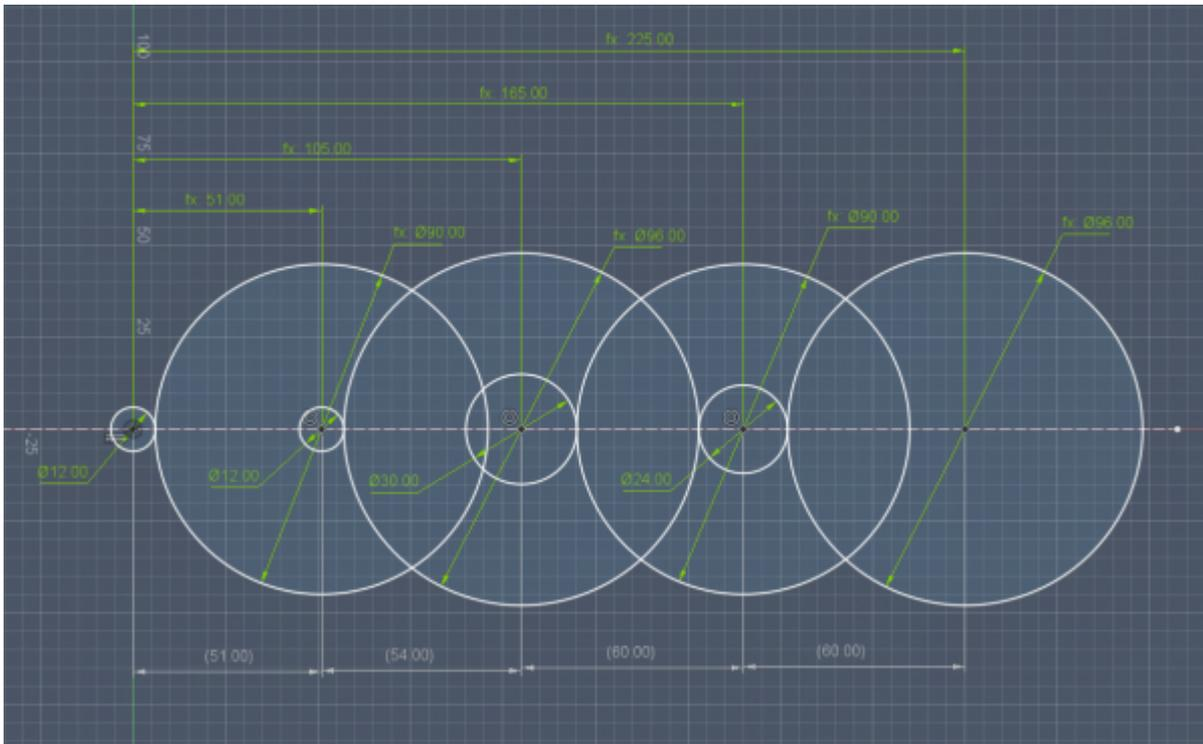
So then working backwards with the gear pitch<sup>5)</sup>, through trail and error I managed to get to this solution in a straight line.
