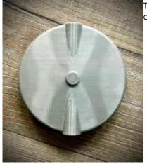
The pendulum weight design is 100mm in diameter and hollow and filled with sand to create the weight. The design linked here fully filled is about 140g.
