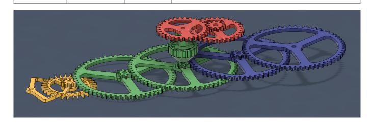
So this is a coloured view of the entire drive train with the yellow parts being responsible for generating the seconds, green then stepping that down to minutes and delivering the output to a shaft driving the minute hand. The red gears than steps everything down further by a combined ratio of 12 and driving the hour hand. Lastly the blue gears stepping down everything by another ratio of 56.25 to provide enough power for 10 days.
