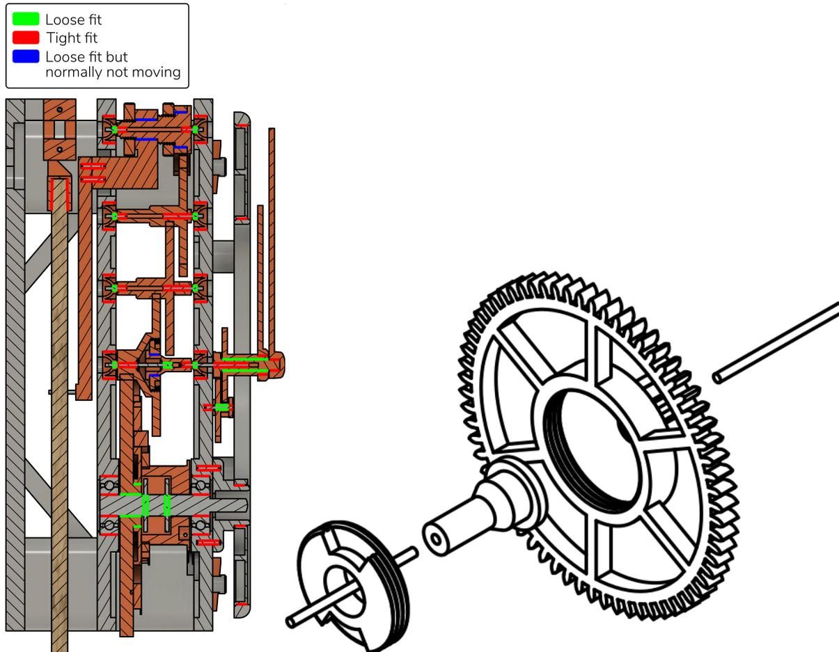
In the section view on the left, right in the middle line where the dials are attached, is the assembled part and to the right the exploded view.
