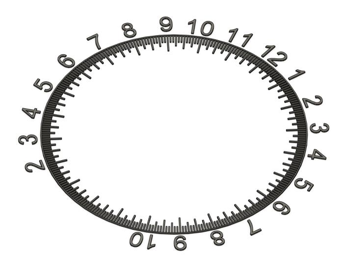
Then create the faceplate on the same layer, extruding downwards to create a thicker body that the parts in step one, for example, the numbers and lines in part one I created is 0.8mm deep, so will be four layers deep with a print height set at 0.2mm. The Faceplate body I extruded to 3mm.
